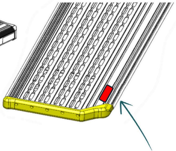
If the serial number sticker cannot be found in this location a serial number 'plate' can be found elsewhere on the step.
