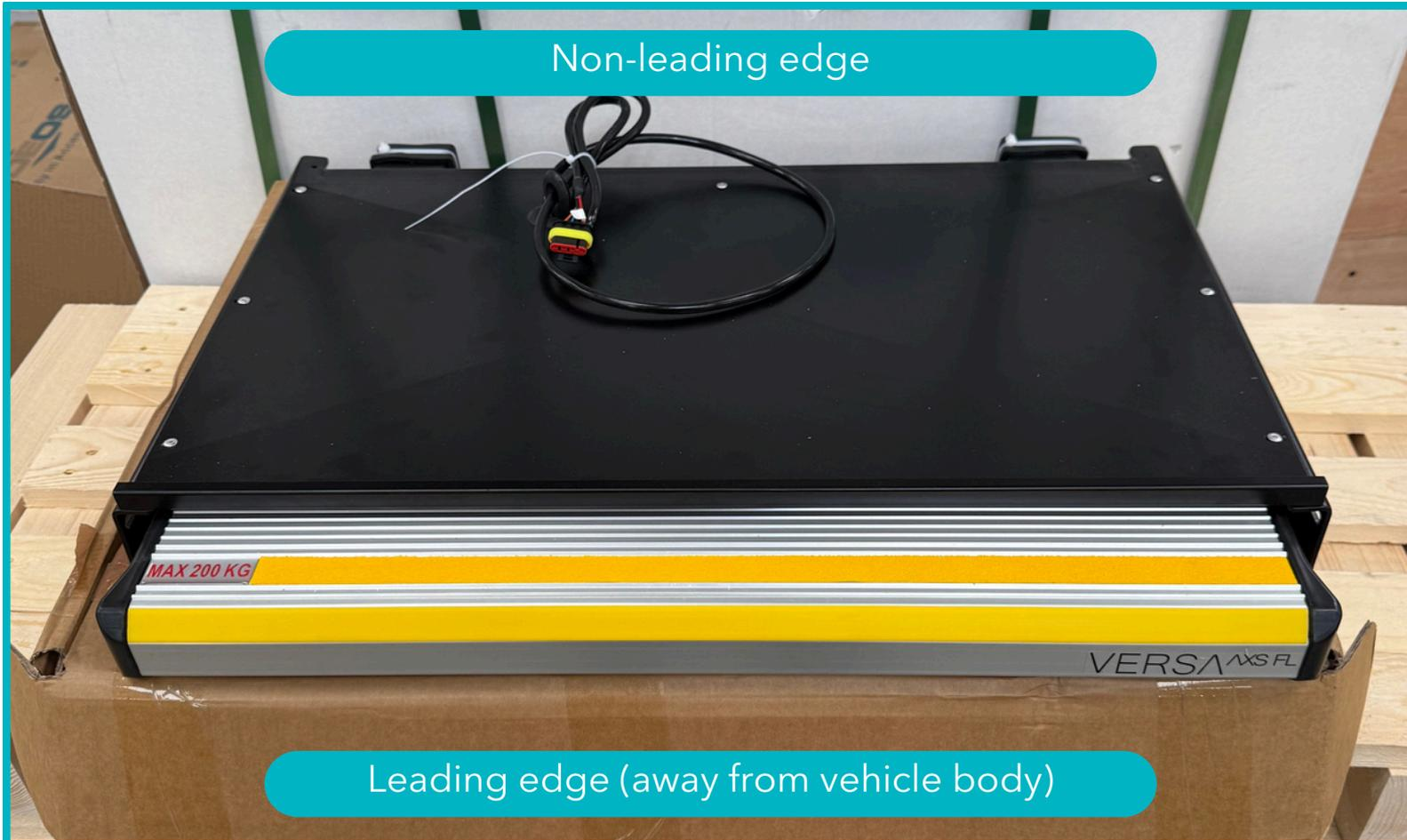
Viewed from rear the step serial number plate is affixed at the back of the step housing
